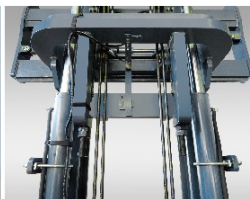
Terminal buffer of lifting
